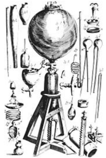
Air pump built by Robert Boyle . Many new instruments were devised in this period, which greatly aided in the expansion of scientific knowledge.
